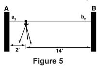
a distance (d<sub>a</sub>)=|a<sub>1</sub> -a<sub>2</sub>|
